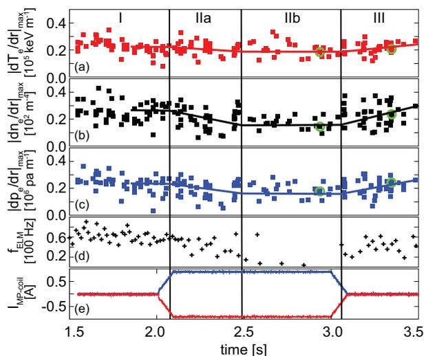
Figure 2: Time traces of the maximal edge gradients of (a)  $T_e$ , (b)  $n_e$  and (c)  $p_e$  together with (d) the ELM frequency and (e) the current of an upper (blue line) and corresponding lower (red line) MP coil of discharge #26078; time points of profiles in Fig. 1 marked by green circles
