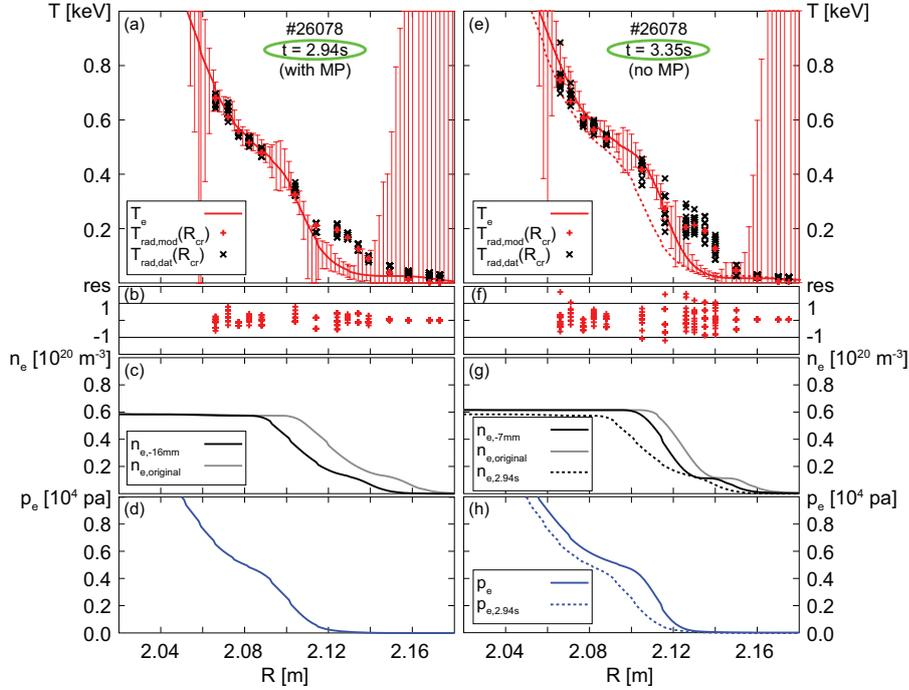
Figure 1: (a,e) Edge  $T_e$  profiles (red lines) together with the modelled (red pluses) and measured (black crosses)  $T_{\text{rad}}$  values at the positions of their cold resonance and (b,f) the corresponding  $T_{\text{rad}}$  residual values, (c,g) shifted (black) and original (grey)  $n_e$  profiles and (d,h)  $p_e$  profiles of discharge #26078 at  $t = 2.94$  s (left) and  $t = 3.35$  s (right); the dashed lines on the right replicate the profiles at  $t = 2.94$  s
