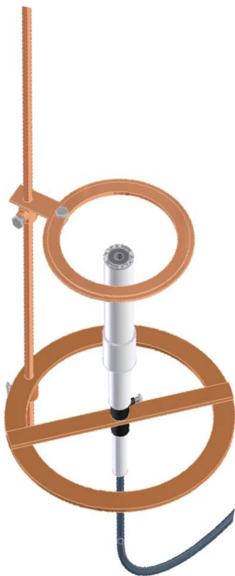
Fig. 1. Photo of the simple experimental set-up of the hollow cathode.
