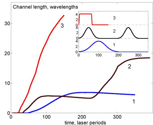
Figure 1: Temporal dynamics of the channel length  $L(t)$  in a plasma. The pulse shapes are shown in the insert.
