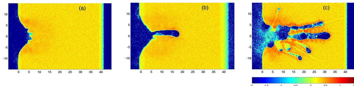
Figure 2: Spatial distribution of plasma density: (a) a single pulse  $\tau_p = 50 T_0$  at the time instant  $t = 230 T_0$ ; (b) two pulses  $\tau_1 = 25 T_0$  with the time delay  $T_{\text{delay}} = 200 T_0$  at the time instant  $t = 405 T_0$ ; and (c) a flat top pulse  $\tau_2 = 58.9 T_0$ ,  $\tau_f = 5 T_0$  at the time instant  $t = 144 T_0$ . The spatial coordinates are scaled in the vacuum wavelengths  $\lambda_0$ .
