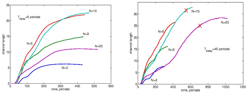
Figure 3: Temporal evolution of the channel length in function of the number  $N$  of pulses for  $T_{\text{delay}} = 5T_0$  (a) and  $T_{\text{delay}} = 40T_0$  (b). The pulse amplitude  $a_m = 4$ . Red crosses mark the moments when the layer is bored through.
