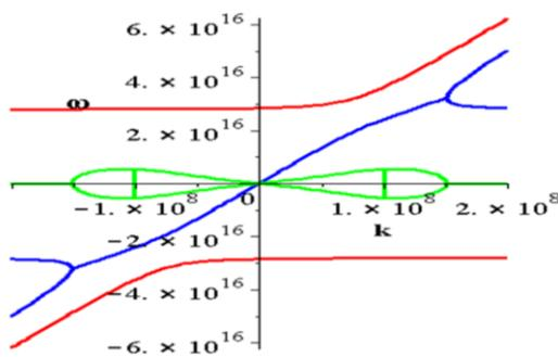
Figure 1. Two-stream dispersion solution for a beam-plasma system with background plasma density of  $10^{29} \text{m}^{-3}$ , electron beam density of  $10^{28} \text{m}^{-3}$  and electron beam energy of 1MeV. The red line is the real root for the plasma contribution to the dispersion, the blue line is the real component from the beam and the green line is the imaginary component of the solution from the beam.
