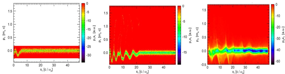
Figure 4a, b, c. Phase space plots of axial momentum against axial position of background plasma electrons at  $t = 9.80, 39.20$  and  $177.50\omega_{pe}^{-1}$  respectively.
