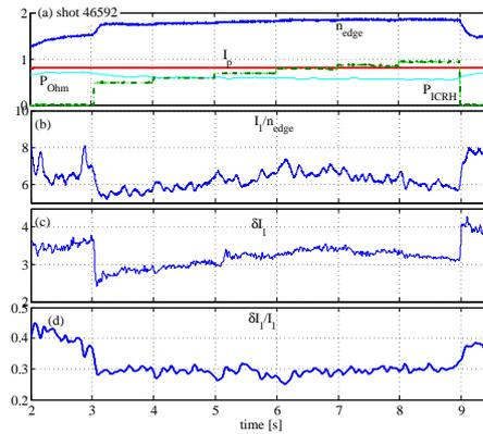
Figure 1: In (a) we inserted the plasma current,  $I_p$  in MA in thick solid line, the edge plasma density  $n_{edge}/10^{19} \text{ m}^{-2}$ , the ohmic power,  $P_{Ohm}$  in MW and the dash-dotted line the ICRH power  $P_{ICRH}$  in MW. In (b), we plot the average  $I_{sat}$  normalized to the edge plasma density. In (c), the standard deviation of  $I_1$  is plotted as a function of time and in (d) the normalized level of fluctuations is shown to decrease from about 0.4 to 0.28.
