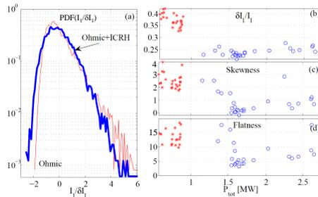
Figure 2: The PDF of the ion saturation current normalized to the standard deviation is plotted in (a) for ohmic and ICRH plasmas. In (b), (c) and (d) respectively we have the normalized level of fluctuations, the skewness and the flatness factors.
