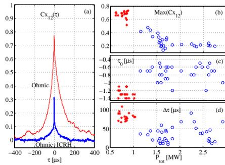
Figure 3: The cross-correlation coefficient between probes 1 and 2,  $Cx_{12}(\tau)$  as a function of time  $\tau$  is plotted in (a). In (b), the maximum of  $Cx_{12}$  is plotted as a function of the total power. In (c), we illustrate the time corresponding to the maximum amplitude  $\tau_0$  as a function of  $P_{tot}$ . (d), the width of  $Cx_{12}$ , denoted by  $\Delta\tau$  as a function of  $P_{tot}$ .
