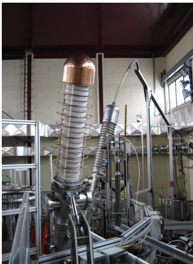
Figure 4. Photo of the new second HIBP injector (at the foreground), and the first one with high voltage connection (background).
