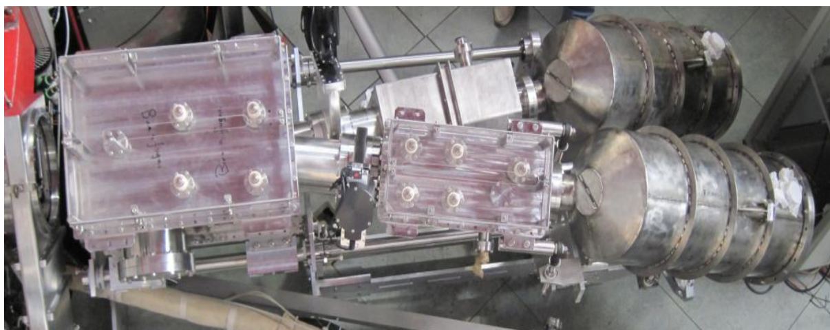
Figure 5. Photo of the two energy analyzers with the secondary beamlines with correcting electrostatic plates.
