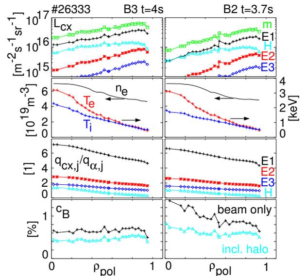
**Fig.3:** Profiles for impurity emission and derived quantities measured during #26333. left: beam 3, right: beam 2. top row: measured radiance of the boron  $n=7-6$  transition (m, green) and calculated contributions from halo and beam neutrals. second row:  $n_e$ ,  $T_e$ , and  $T_i$ . third row: CX photons per  $D_\alpha$  photon for  $c_B=1$ . bottom: derived boron concentration with and without considering the halo neutrals.
