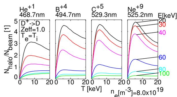
**Fig.4:** Ratio of halo to beam induced CX-lines as a function of beam energy and plasma temperature.
