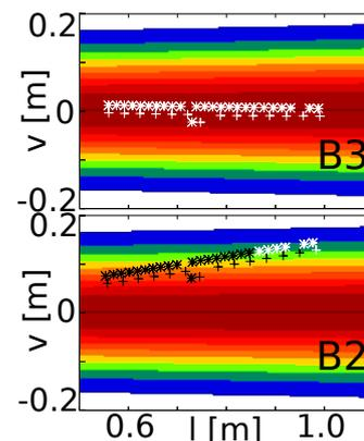
**Fig.1:** Position of the closest approach of LOS and beams (crosses for BES, stars for CXRS) and beam density cross-section.
