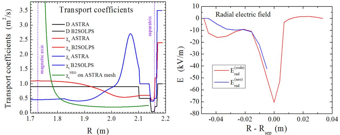
Figure 5. Transport coefficients used in Figure 6. Radial electric field at equatorial midplane and neoclassical formula for AUG.
