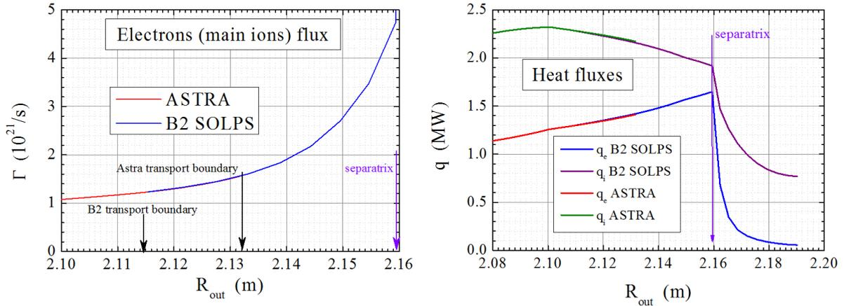
Figure 3. Calculated total particle and energy fluxes through flux surface in AUG.
