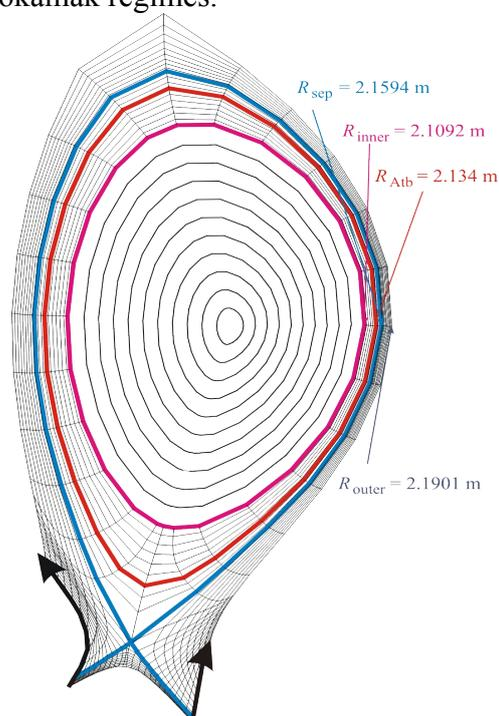
Figure 1. Computational domains for ASTRA and B2SOLPS codes. Blue line represent a separatrix, red one – outer boundary of ASTRA domain, magenta one – inner boundary of B2SOLPS domain.
