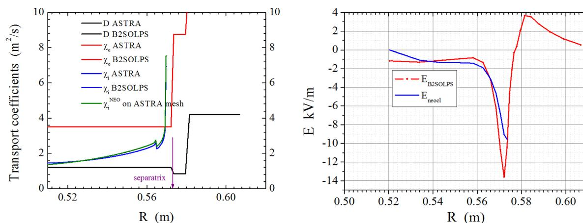
Figure 8. Transport coefficients used in Figure 9. Radial electric field at equatorial midplane calculations for Globus-M shot #29076.
