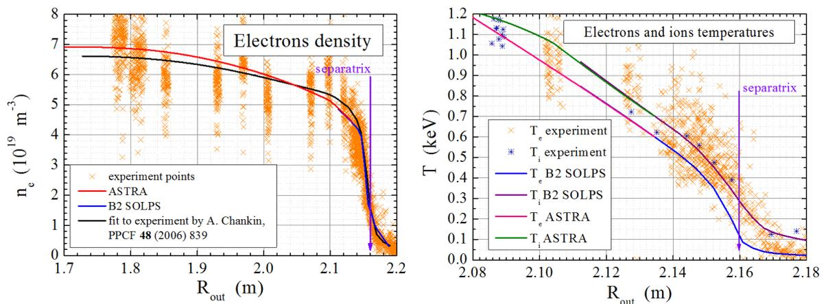
Figure 2. Calculated density and temperature profiles at equatorial midplane in AUG.
