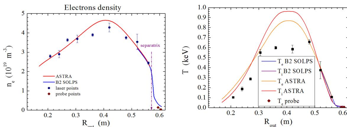
Figure 7. Resulting density and temperature profiles for Globus-M shot #29076.
