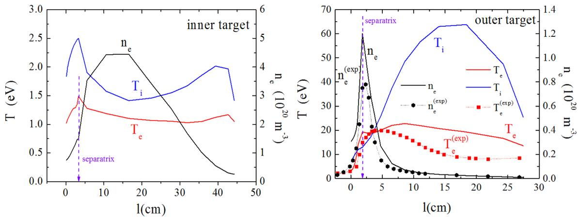
Figure 4. Temperature and density profiles at targets calculated for ASDEX-Upgrade. Distance is measured along plates in poloidal direction as shown by black arrows in Fig. 1.
