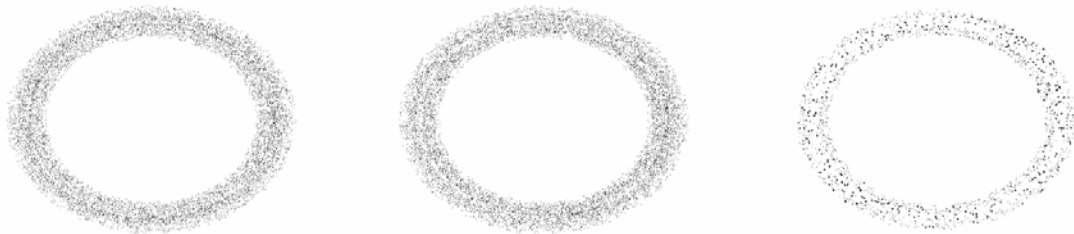
Fig. 3: Poincaré sections for 20eV ions at potential amplitude 0V (left), 0.03V (middle) and 5V (right).
