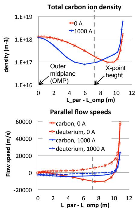
Figure 4: Carbon ion density and carbon and deuterium parallel flow speeds as a function of distance along a field line from the outer midplane to the outer divertor target on the 2-mm flux surface.
