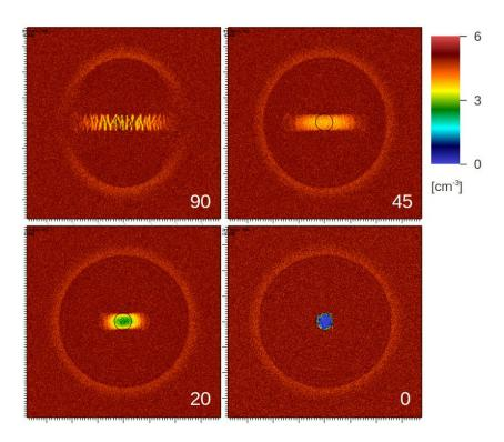
Figure 1: Proton number density in the yz-plane at t = 200 s for an IMF direction of 90, 45, 20, and 0 degrees away from the image normal (solar wind direction). The plane of the IMF is horizontal. The black circle show the outline of the initial low density region of radius 1730 km (representing the Moon).
