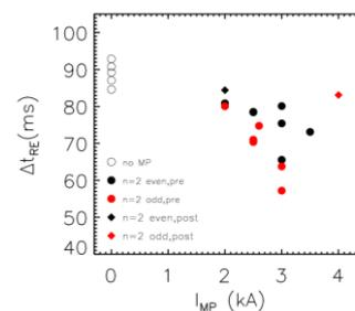
**Figure 3.** Runaway beam duration ( $\Delta t_{RE}$ ) as function of amplitude ( $I_{MP}$ ) of odd and even parity  $n=2$  MP, applied before or after disruption.
