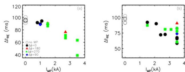
**Figure 2.** Runaway beam duration ( $\Delta t_{RE}$ ) as function of MP amplitude ( $I_{MP}$ ) for different phasing values (colors/symbols). In (a) MPs have been applied before the disruption, in (b) after.
