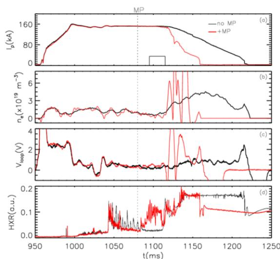
**Figure 1.** Example of disruptive discharges in COMPASS without (black, #15774) and with (red, #15775) MP applied; from the top: (a) plasma current, (b) electron density (oscillations in the red trace after disruption are caused by fast variations of the radial RE beam position and of other signals), (c) loop voltage and (d) HXR radiation. MP pulse starts at the time corresponding to the vertical dotted line and the Ar injection is represented by a rectangle in the top panel.
