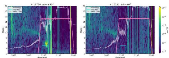
**Figure 4.** Time-frequency spectrogram from Mirnov coil signal ( $T$ ) when  $n=2$  MPs with odd (left) or even (right) parity are applied before disruption. White line corresponds to HXR signal, pink to the MP amplitude and cyan to Ar injection.
