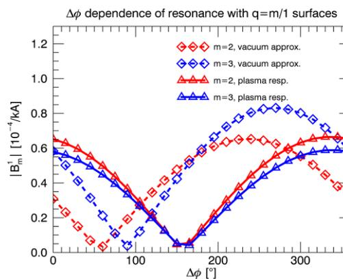
**Figure 5.** Perturbed field at resonant positions  $q = 2$  (red) and  $q = 3$  (blue) in vacuum (diamonds) and with plasma response (triangles) as function of the phasing for  $n = 1$  MP.
