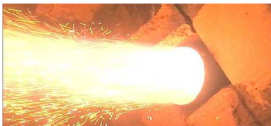
Fig. 5 Pulverized coal flame of plasma arc burner
