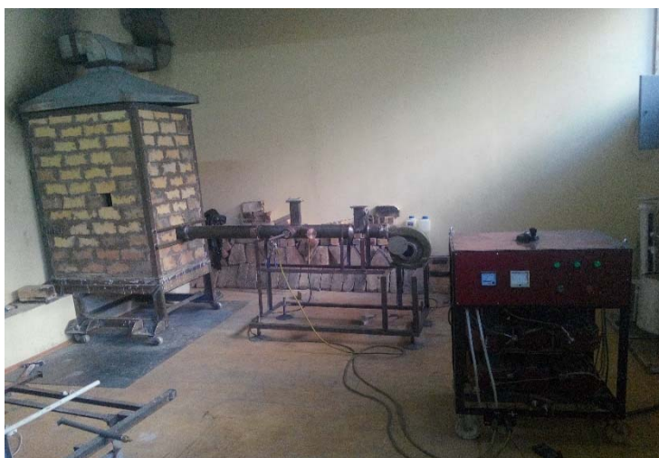
Fig.4 Plasma arc burner laboratory mock-up
