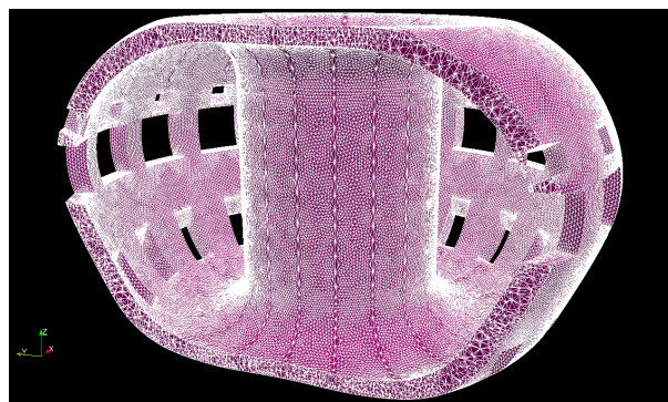
Figure 4: Mesh of a low feature vessel.
