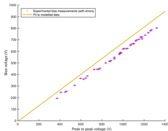
Figure 2: *Electrode bias in experiment and simulation. All model data points lie on the fitted line.*
