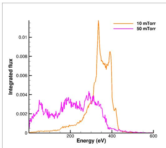
Figure 3: *IEDFs for 10 and 50 mTorr at an RF potential of 400 V*
