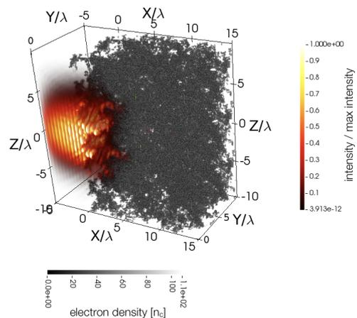
Figure 1: Nanostructured foam irradiated at  $a_0 = 5$ . Electron density is shown in greyscale, while EM field intensity is shown in color scale.
