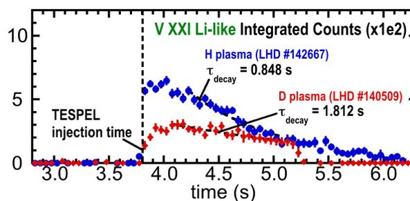
Fig. 1 Temporal evolution of Vanadium Li-like integrated counts measured with a VUV spectrometer.
