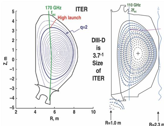
Fig. 1. Cross-sections of ITER and of a DIII-D ITER Baseline Scenario discharge showing the launch of rays (170 GHz  $1 \cdot f_{ec}$  and 110 GHz  $2 \cdot f_{ec}$  respectively) to drive co-ECCD at  $q=2$ .
