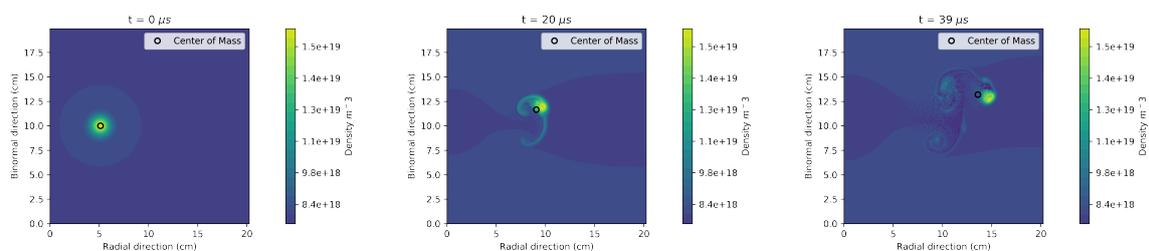
Figure 1: Filament density plots exhibiting typical radial propagation.
