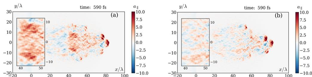
Figure 1: 2D simulation of the longitudinal field distributions created by a tightly focused 10 PW laser pulse of FWHM duration  $t_{\text{pulse}} = 150$  fs, propagating in a plasma (a) with and (b) without friction.
