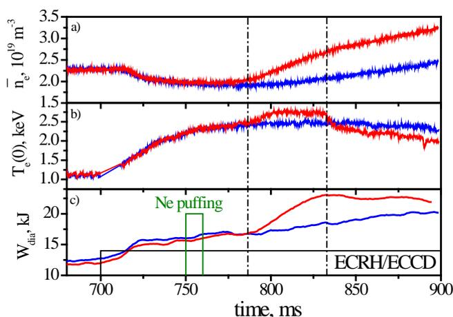
Figure 1. Time evolution of the electron density (a), central electron temperature (b) and plasma energy content (c) in similar T-10 discharges with (red curves) and without (blue curves) Neon puffing. Time and duration of Ne puffing and ECRH/ECCD are presented in subplot (c).
