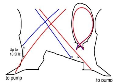
Figure 1 Strike point sweeping perturbs the recycled particle fluxes in the vicinity of the strike points as well as the divertor conditions in general thus affecting upstream SOL profiles and core fuelling. The main plasma shape as well as other heating and fuelling parameters are kept constant.
