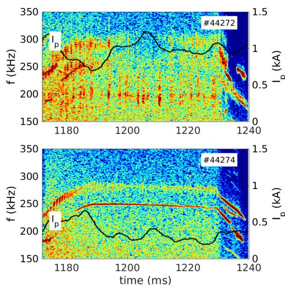
Figure 1: Spectrogram of magnetic fluctuations with (bottom) and without ECCD (top).
