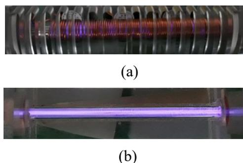
**Fig. 2.** Photographs showing the stable DBD plasma from air gas grounded with (a) coiled electrode and (b) surrounded with water.
