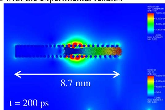
Figure 1: Chromatic focusing phenomenon reproduced by numerical simulation (SOPHIE code).
