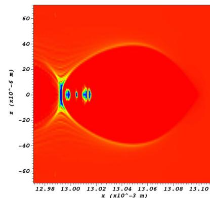
Figure 1: Density distribution of electrons from a simulation where the driving beam charge is 2.4 nC and the density down-ramp is  $L_n = 1.5$  cm long.
