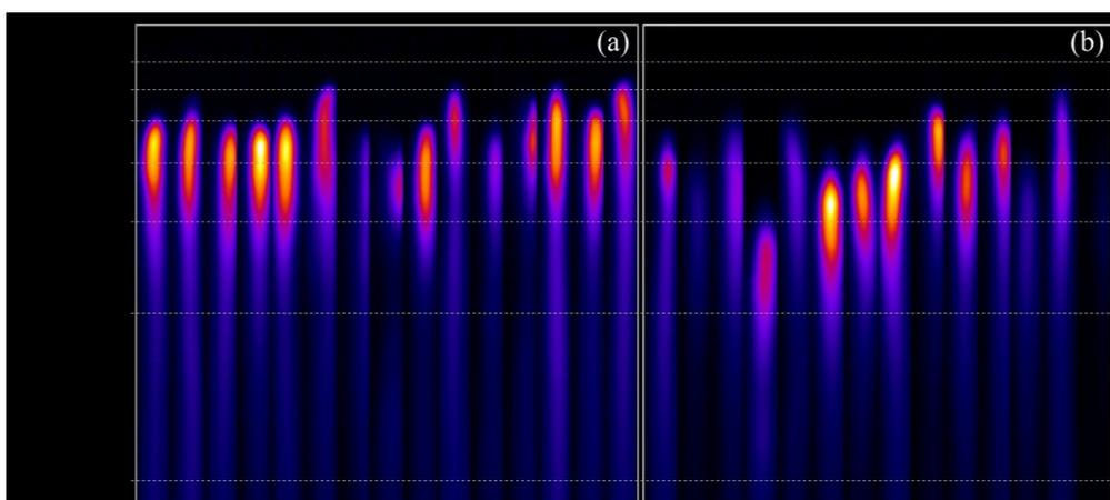
**Fig. 1.** Images of spectrally dispersed electron beam produced from 2.3mm long helium gas jet plasma at constant plasma density in series of consecutive shots (a) when the elliptically shaped laser beam with major axis along laser polarization was used, and (b) when a laser beam without shaping was applied with appropriately reduced energy to maintain similar laser strength parameter.
