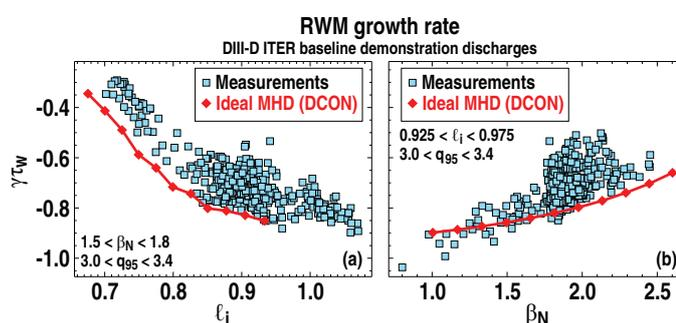
Figure 1: Comparisons of the (a)  $\ell_i$  and (b)  $\beta_N$  dependencies of the normalized RWM growth rate  $\gamma\tau_w$  inferred from plasma response measurements (squares) with predictions of the linearized, ideal MHD, resistive wall dispersion relation (diamonds).
