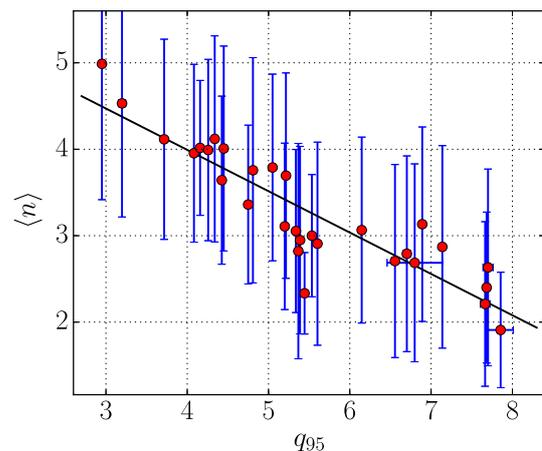
Figure 1: Average toroidal mode numbers  $\langle n \rangle$  of mode structures during the ELM crashes of 30 ASDEX Upgrade H-mode discharges against the edge safety factor  $q_{95}$ .
