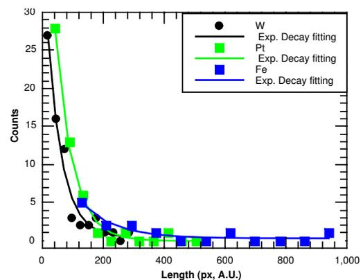
Figure 1: *Distance distribution for the peaks and valleys of exploding wire plasmas.*
