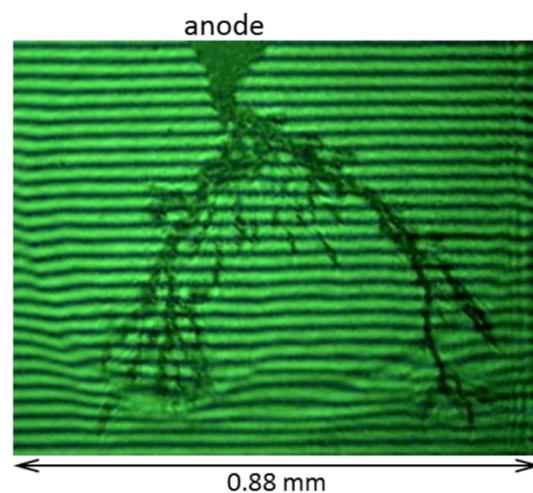
Figure 1: Typical interferogram of the pulsed discharge in water media, taken from [1].
