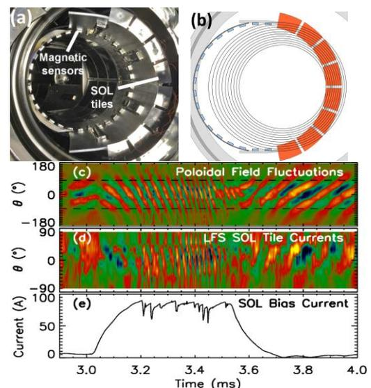
Magnetic sensors and SOL current tiles pictured in (a) measure MHD activity with poloidal and toroidal resolution. Sensor layout and SOL flux surfaces for a discharge with SOL biasing are shown in (b). Tile current (c) and magnetic (d) fluctuations versus poloidal angle show rotating MHD responding to applied SOL current (e).
