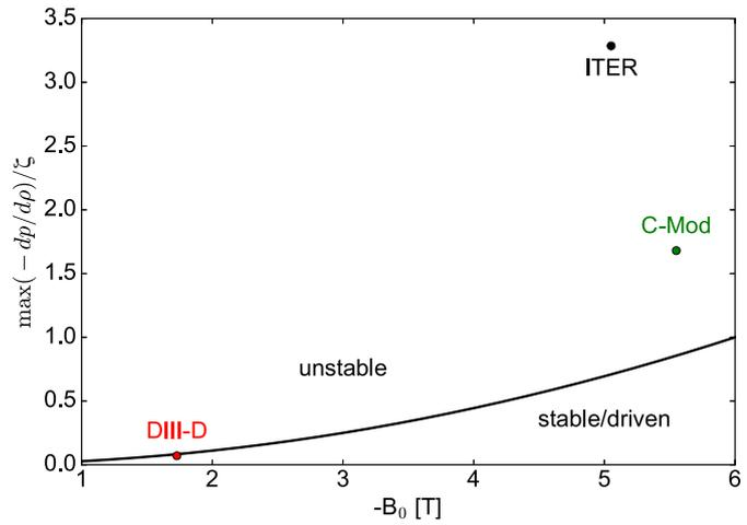
Figure 1: Onset of helical cores for an ITER mock-up discharge (15 MA, H-mode), compared to 3-D reconstructed DIII-D and C-Mod discharges. The y-axis is normalized so that the thresholds for all machines coincide, with:  $\zeta_{DIII-D} = 2.545$ ,  $\zeta_{ITER} = 0.5$  and  $\zeta_{C-Mod} = 0.145 \cdot 10^6 Pa$ .
