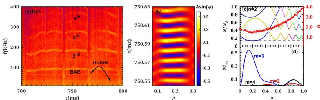
Fig.1 (a) Stationary i-BAE and (b) the corresponding mode structure detected by microwave reflectometer. (c) The  $q$  profile and Alfvén continuum for stationary i-BAE with  $n=2$ . (d) The radial mode structure given by the AMC.
