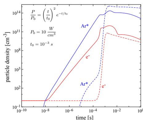
Figure 1: *Electron and argon metastable densities with (continuous lines) and without (dashed lines) superelastic collisions in the Boltzmann equation.*
