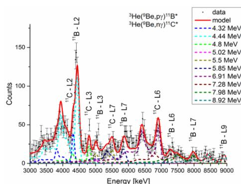
Figure 1. Gamma-ray spectrum from reactions between fast <sup>3</sup>He ions and <sup>9</sup>Be impurities in 3 ion ICRH experiments at JET. A detailed analysis of the complex gamma-ray spectrum born in these reactions resolves the individual contributions to the emission, which are used to determine the <sup>3</sup>He ion energies for comparison with models.
