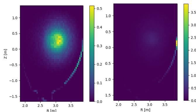
Figure 1: HALO predictions of TRANSP fusion product numbers in equilibrium (left) and with the fishbone (right). Calculated losses are completely due to FLR
