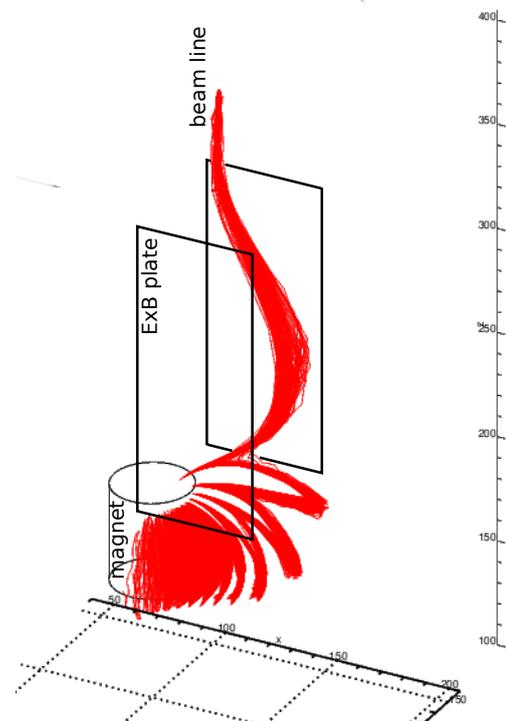
Figure 1: Simulated trajectories of a finite-temperature positron bunch being losslessly drift-injected into a dipole trap.
