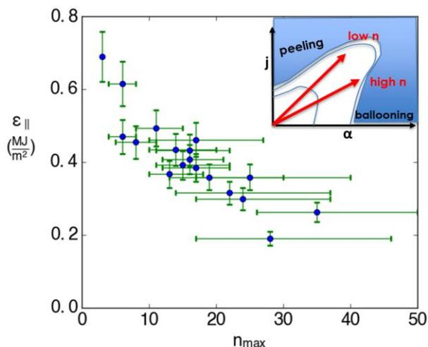
Figure 1 Inverse proportionality between linear mode number with the highest growth rate and peak parallel ELM energy density for type-I ELMy plasmas
