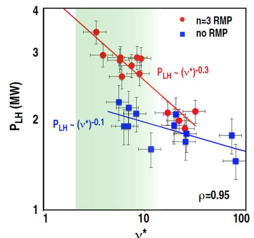
Fig. 1: L-H transition power threshold  $P_{\text{LH}}$  vs. collisionality  $\nu^*$  ( $\rho = 0.95$ ) without and with applied n=3 RMP ( $3.3 \times 10^{-4} \leq \delta B/B \leq 4.6 \times 10^{-4}$ ). The expected ITER L-mode edge collisionality range is shaded.
