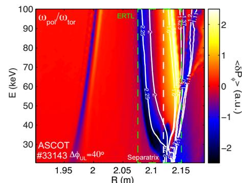
Fig 1.  $\langle \delta P_\phi \rangle$  structures in the presence of a  $\Delta\phi_{UL}=40^\circ$  magnetic perturbation configuration overlapped with matching orbital resonances ( $\omega_{pol}/\omega_{tor}$ ). Black-blue areas represent outwards transport while yellow-white means inwards transport.
