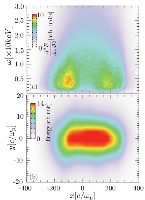
Figure 2: Spectrum of radiation emitted by the arbitrarily chosen 500 trapped accelerating particles: (a) radiation frequency distribution on x axis ( $y=0$ ), and (b) radiated energy distribution in x-y plane. The spectrum is obtained at  $z = 5500c/\omega_p$ .
