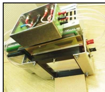
Fig. 2b: Structure of the Prototype-II T-GEM X-ray detector [3].
