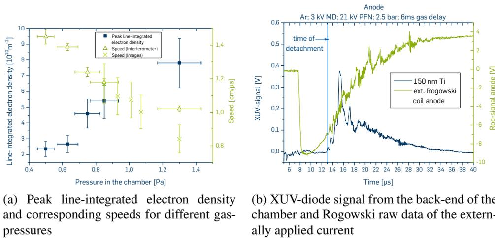
Figure 2: Current measurement in the apex and XUV measurement with line-of-sight on the anode
