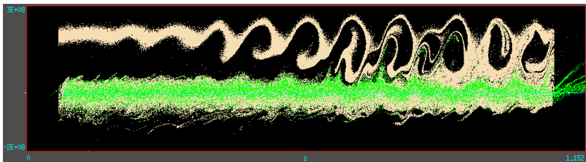
Fig 2 - Z-momentum against z of all particles in the simulation after 70ns (orange=beam electrons, green=plasma electrons, blue=plasma ions)
