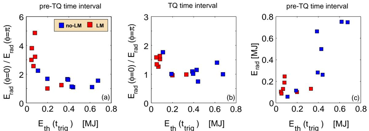
**Figure 2.** (a) Values of the toroidal asymmetry factor,  $AF$ , versus thermal energy of the target plasma during the (a) pre-TQ and (b) TQ phase. (c) Energy radiated during the pre-TQ as measured by the foil bolometers versus thermal energy of the target plasma.
