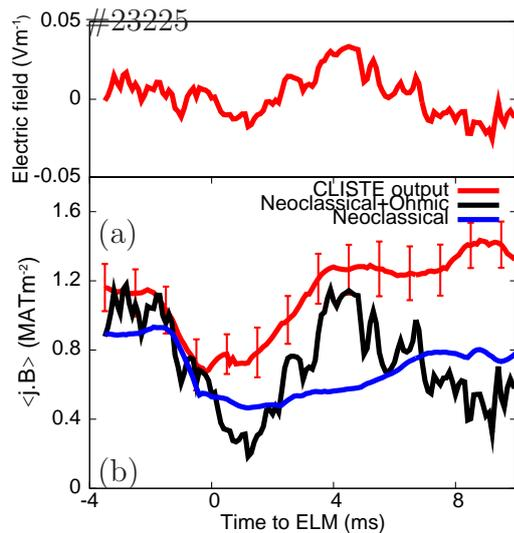
**Figure 4:** (a) shows the electric field calculated at the peak bootstrap position using a resistive current propagation model. (b) shows the flux surface averaged current density from CLISTE (red),  $\langle j_{neo} \cdot B \rangle$  (blue) and  $\langle j_{neo} \cdot B \rangle + \langle j_{ohmic} \cdot B \rangle$  (black).
