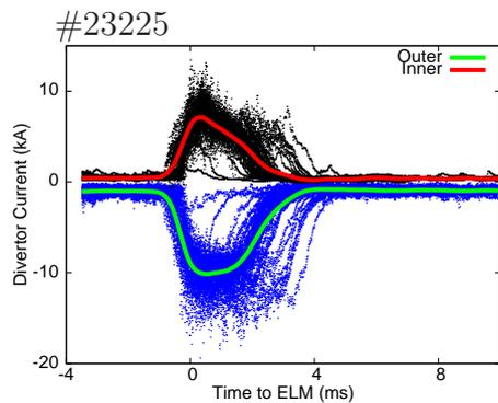
**Figure 2:** ELM averaged divertor currents. The currents are measured as flowing into a divertor tile.
