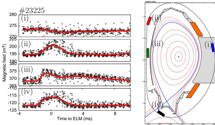
**Figure 1:** (i)-(iv) show the recorded magnetic signals at various points around the torus, as indicated in (b), which shows the equilibrium at -3 ms to an ELM.
