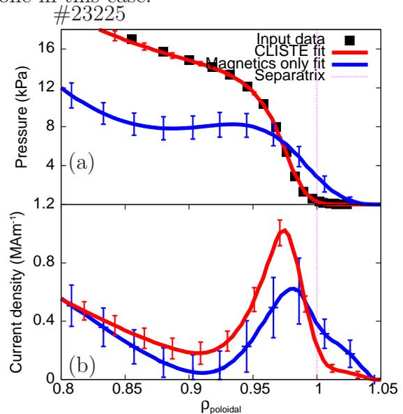
**Figure 3:** (a) Pressure profile. (b) current density profile. The blue line denotes a fit made only with magnetics constraints, while the red line is the fit using a prescribed pressure profile. Black boxes represent input data points. Error bars are 1 sigma confidence bands.
