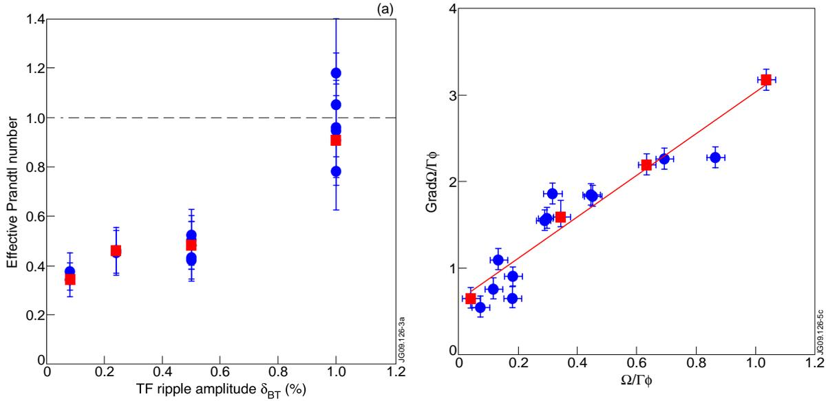
**Figure 2a:** (left) Effective Prandtl number for various discharges as a function of TF ripple. **2b:** (right) The normalised momentum density gradient versus the normalised momentum for the same discharges. The four discharges shown in figure 1 are indicated by the red squares.
