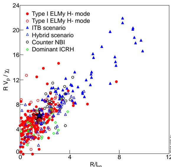
**Figure 3:** The normalised momentum pinch from the rotation database estimated using eq. (3) under the assumption the ion and momentum diffusivities are equal. The black star shows the value of normalised pinch derived from the analysis of the TF ripple experiments shown in figure 2b.
