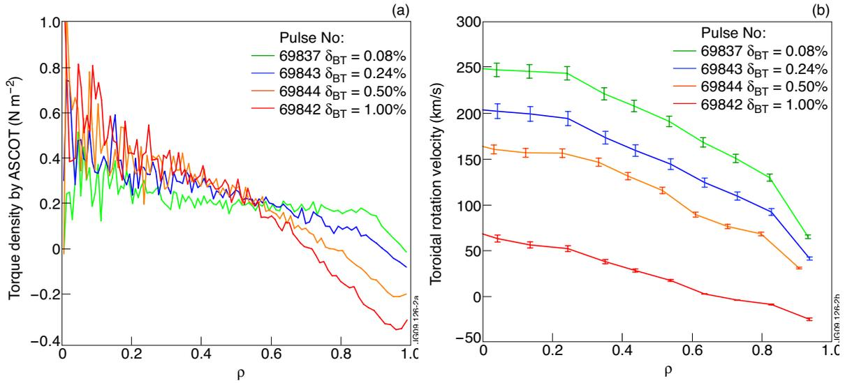
**Figure 1a:** (left) Torque deposition profiles for 4 identical discharges, however, with increasing levels of TF ripple. **1b:** (right) The changes in the toroidal rotation profiles for the same 4 discharges, as measured by Charge Exchange Spectroscopy.
